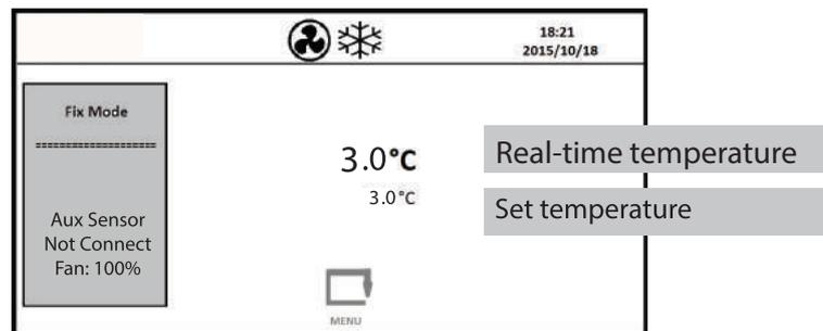
Figure 6: Real-time and set temperatures displayed in the main Menu
