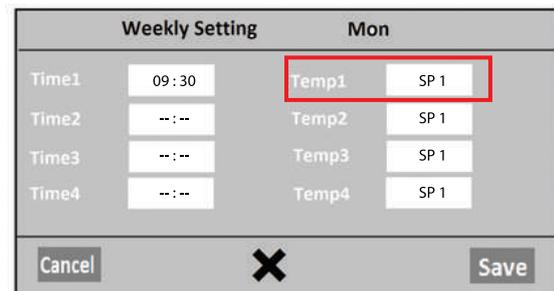
Setting Temp 1: choose one of set temperatures in Fix Mode (SP1 or SP2) by ▲ or ▼ buttons. Then, push ▶ button.
